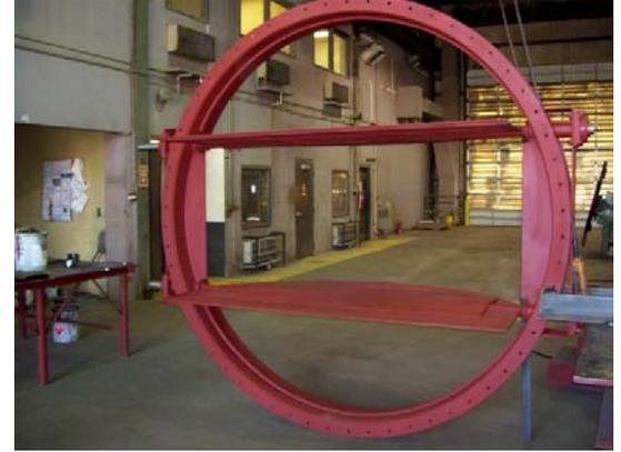
This new butterfly damper was fabricated at our Alabama facility for use at the same North American steel mill. The butterfly damper included a modulating actuator which was tested for proper operation before shipping.
